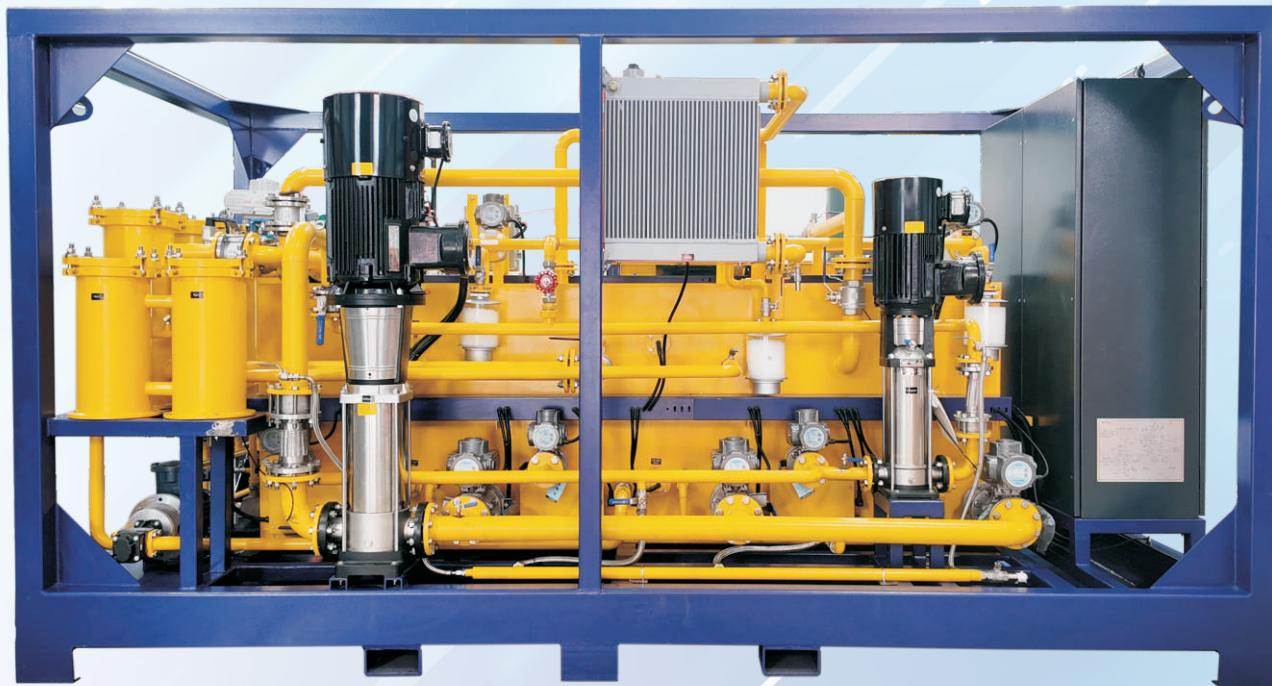
The pipeline flushing equipment (flushing pump flushing equipment) is designed to filter out contaminants generated during pipeline construction (installation), improve system cleanliness, and maintain oil cleanliness within the contamination tolerance of key hydraulic components in the system. This ensures the reliability of the hydraulic system and the service life of components, serving as a necessary measure to eliminate or minimize early equipment failures.
